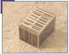
**Stacked, packed.** Chip-stacking technology facilitates extreme miniaturization of superconducting electronics, potentially enabling them to eliminate bottlenecks currently plaguing Internet and telecommunications traffic. Using this technology, Irvine Sensors is packaging SuperRouter<sup>™</sup> switch electronics into a space comparable to the size of a fiber-optics cable.
